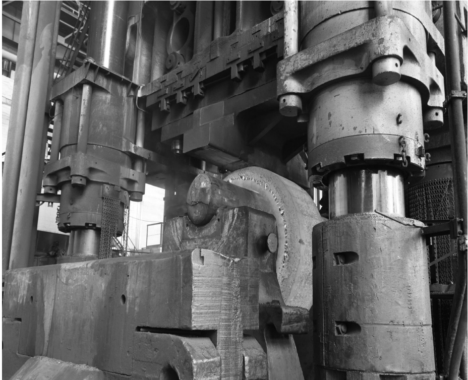
Figure 8.1 – Rolling-of the ring after the upsetting
