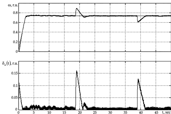
Fig. 4. Transition function for the speed in relative units and corresponding absolute value of the dynamic error (only one discrete time equalizer)
