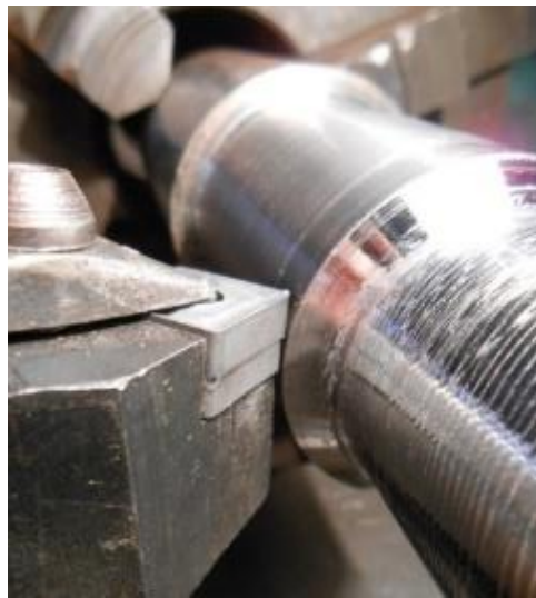
Figure 2.4 - The position of the insert relative to the processed part in determining the resistance to failure and wear under contact load on lathes
