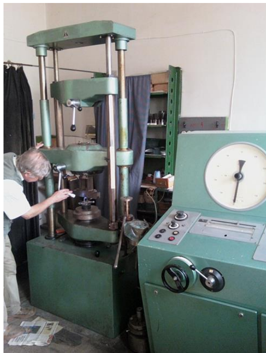
Figure 3.5 - Testing on a ZD-40 hydraulic machine
