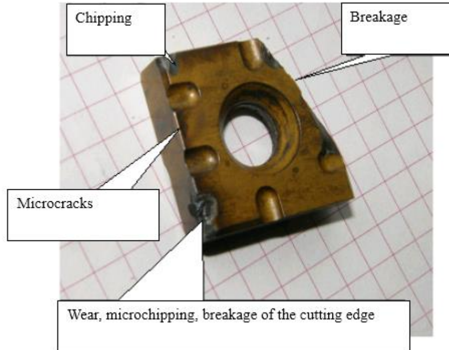
Figure 1.6 - Types of damage and destruction of indexable inserts
